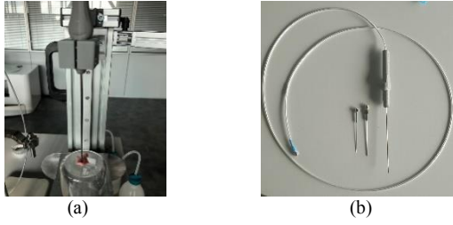
Fig. 1. Measurement set-up: (a) probe with the in vitro rat skin sample, and (b) three probes with 0.5mm, 0.9mm and 2.2mm diameters from left to right.
